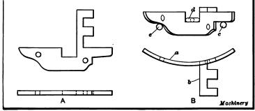
Fig. 12. Blank Before and After Bending Operation
